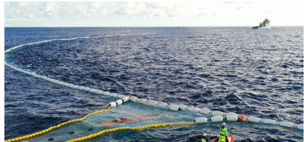
Figure 15: Ocean Cleanup system
